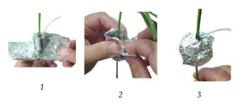
To provide the firm positioning of a sensor on stems with diameter below 4 mm for SF-4z and 8 mm for SF-5z, insert a foam-rubber bar into the internal empty part of a sensor as it is shown below
