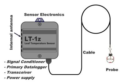
The probe is connected by a standard 1 meter cable to the waterproof box with electronics, which combines signal conditioner, primary datalogger, RF 2.4 GHz transceiver, and power supply (3xAA Alkaline batteries).
