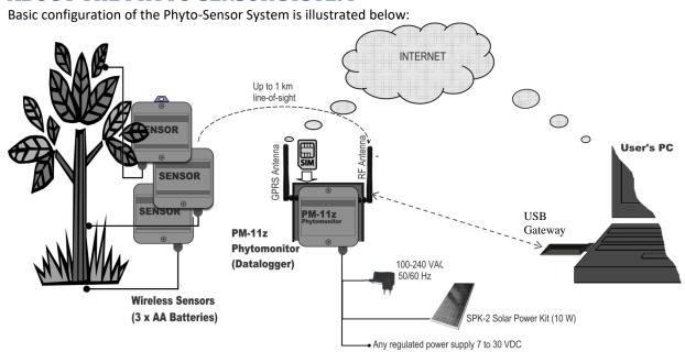
The System hardware includes a variety of wireless sensors for plant and environment, the data logging PM-11z Phytomonitor, USB Gateway, and several optional communication and powering accessories.
