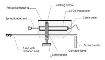
The probe is connected by a standard 0.5-meter cable to the waterproof box with the signal conditioner inside. A signal conditioner provides excitation of the LVDT and production of standard linear output signal.
