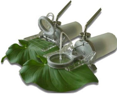
Figure 1. Automatic self-clamping leaf chambers.
