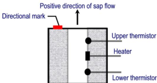
A signal conditioner provides powering of the heater and conditioning of the output signal.
