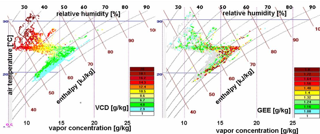
Fig. 5. Scatter plot of VCD (left) and GEE (right) using fog system (n= 15,000).
