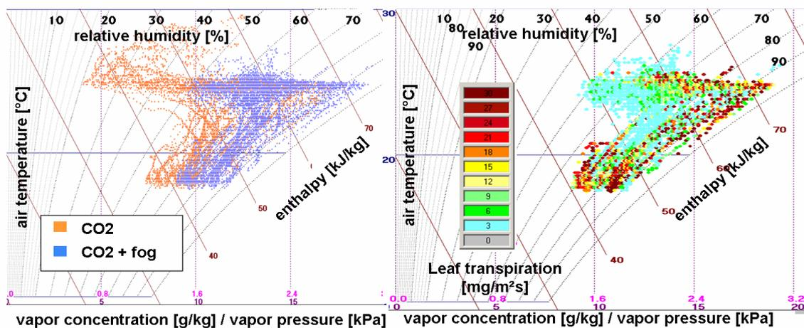
Fig. 6. Scatter plots of CO<sub>2</sub> + fog vs. CO<sub>2</sub> only (left) and leaf transpiration with fog (right).
