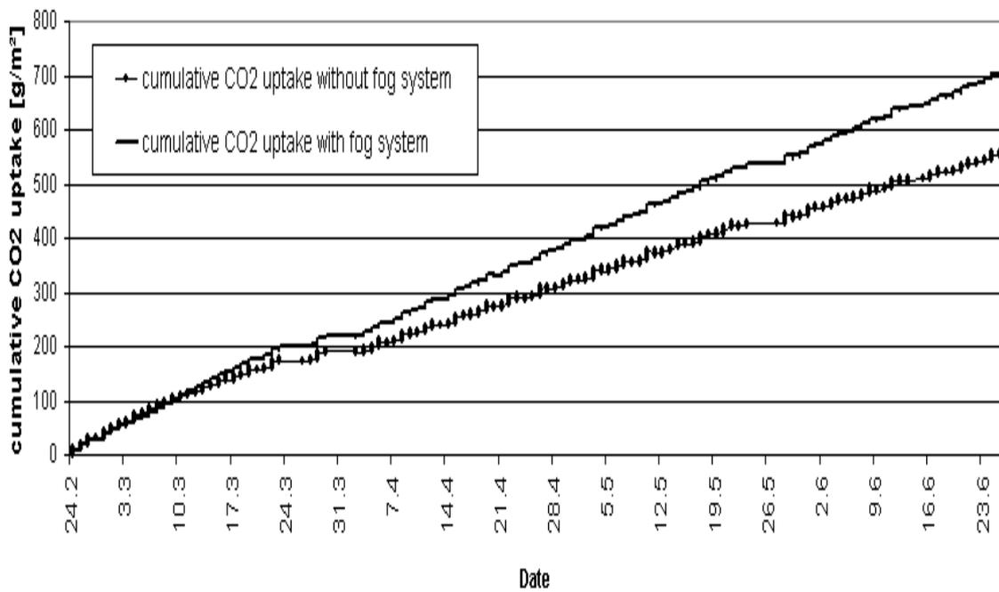
Fig. 4. Comparison of measured cumulative CO<sub>2</sub> uptake between CO<sub>2</sub> enrichment and CO<sub>2</sub> enrichment with fog application.
