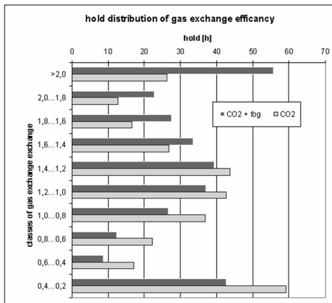
Fig. 2. Hold of gas exchange efficiency at different classes.
