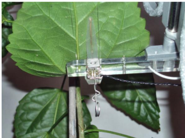
Thermistor should be placed at the lower side of the leaf.
