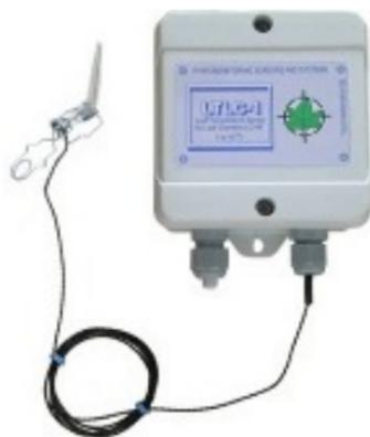
The probe is connected by a standard 1-meter cable to the waterproof box with the signal conditioner inside. Standard cable length between signal conditioner and monitor is 4 meters. Every sensor is tuned and calibrated within the measurement range. The tolerance range is  $\pm 0.08$  °C only.
