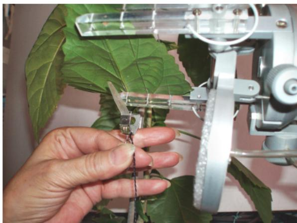
2. Mount the LT-LC sensor on a lower part of a plastic clip between the first and second clamping threads. You may use any of the paired clips.
