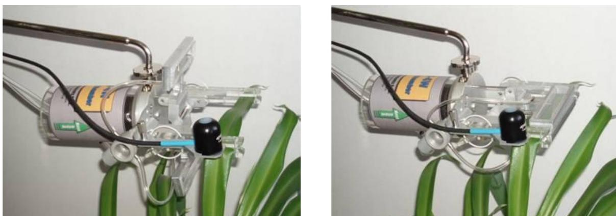
The LC-4W Leaf Chamber has a special plate for mounting optional Quantum sensor for measuring Photosynthetic Photon Flux (PPF) in  $\mu\text{mol}\cdot\text{m}^{-2}\cdot\text{s}^{-1}$ , if necessary.
