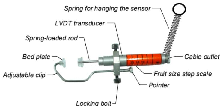
Each FI-XSP sensor is supplied with an electronic signal conditioner and 4-m output cable with the IP67 plug for connecting to the appropriate instrument.
